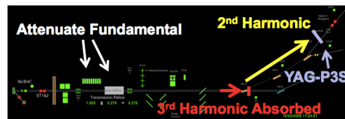
Figure 2: Schematic of the second harmonic measurement. The fundamental is absorbed by attenuators and the third harmonic is absorbed by the beamline mirrors.
