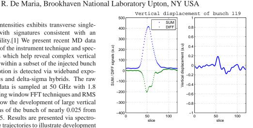
Figure 1: Sum and DeltaY signals from SPS receiver (after equalization). Bunch 119, turn 100 after injection, 26 GeV. The vertical offset is removed in the rightmost plot. Bunch 119 is becoming unstable, as seen in the high-frequency structure. Each slice (sample) is 20 ps.
