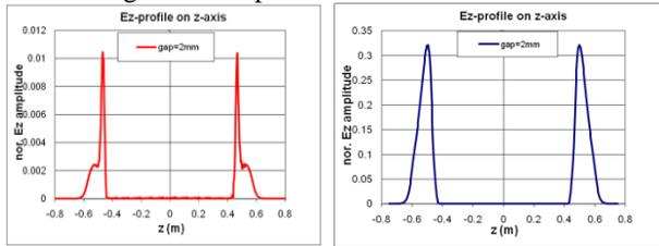
Figure 8: Lowest longitudinal trapped mode  $E_z$ -profiles along the  $z$ -axis using the previous (left) and the current (right) transition designs.
