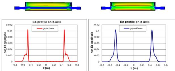
Figure 4: Lowest longitudinal trapped mode E-fields and Ez-profiles along the z-axis for fully inserted jaws (top/bottom left) and fully retracted jaws (top/bottom right) in partial-circular vacuum chamber collimator.
