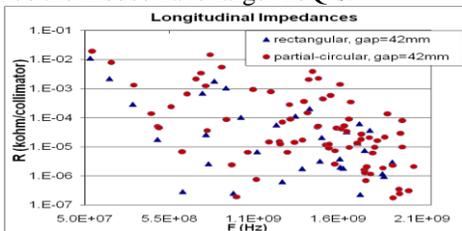
Figure 5: The longitudinal trapped mode impedances for fully retracted jaws in rectangular and partial-circular vacuum chamber collimator designs with previous jaw end and RF contact designs. Form-factors for the beam spectrum are included using 7.55cm bunch length.
