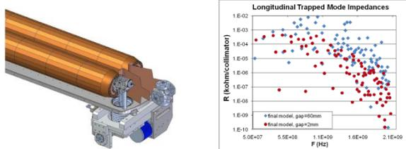
Figure 9: Final collimator (left) and the longitudinal trapped mode impedances (right).
