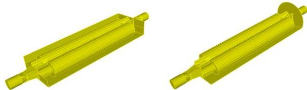
Figure 2: Rectangular (left) and partial-circular (right) vacuum chamber collimator simulation models with the previous jaw end and RF contact designs.
