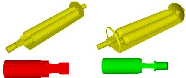
Figure 6: EM simulation models for the partial-circular vacuum chamber collimator with previous (top/bottom right) and current (top/bottom left) jaw end and RF contact designs.
