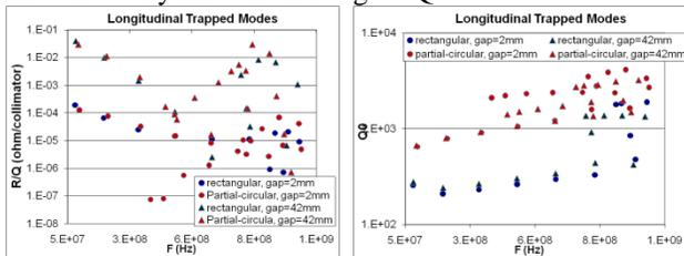
Figure 3: Longitudinal trapped mode R/Q's (left) and Qs (right) with the previous jaw end and RF contact designs in the different vacuum chamber collimators.
