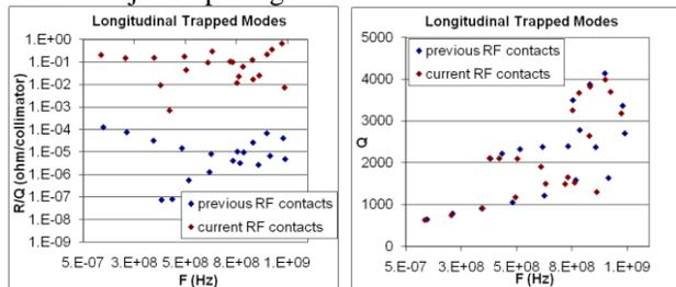
Figure 7: Longitudinal trapped mode R/Q's (left) and Qs (right) in the partial-circular vacuum chamber collimators with different RF contact designs.
