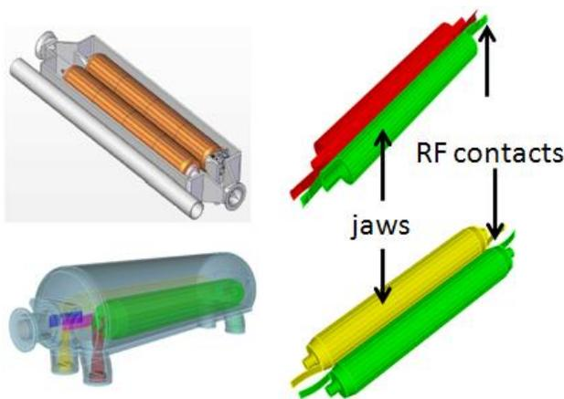
Figure 1: 3D solid models (top/bottom left) and rotatable jaws with RF contacts (top/bottom right) for SLAC previous/current collimator designs.
