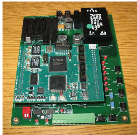
Figure 2: Photograph of the gate driver designed to control 6.5 kV IGBTs in the main stage. The digital control board is stacked to the gate driver board. Dimensions of the gate driver board and the digital control board are 4.5"×5.5" and 3.3"×2.5", respectively.
