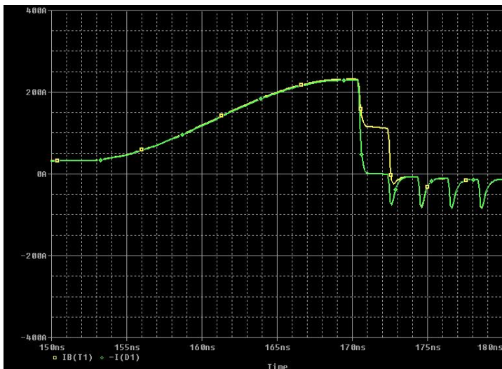
Fig. 7 The DSRD current (green) and the transmission line (L2) current on its end (yellow) vs. time
