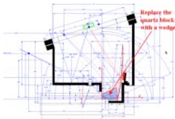
Fig. 8. Geometry of the focusing DIRC with a cylindrical mirror and the wedge (see Fig. 3b) added to see the effect of its inclined surfaces.
