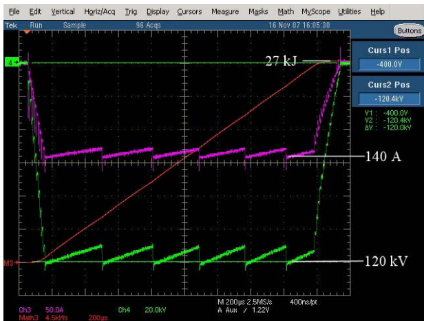
Figure 4: Marx output with coarse flattening, Ch3 is load current, Ch4 is load voltage, and Math3 is load energy.
