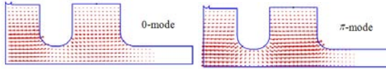
Fig. 3: 0-mode and \pi -mode electric field profiles for the balanced \pi -mode at 2856 MHz.
