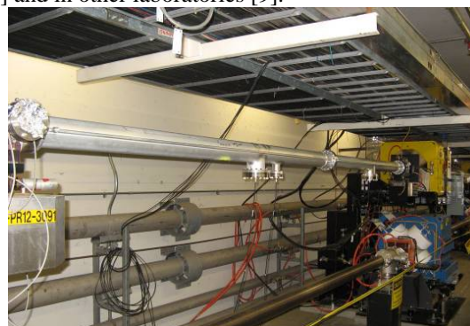
Figure 2. Layout of the installation in PEP-II LER: Groove chambers (left chamber on upper beam line) and smooth chamber (right).
