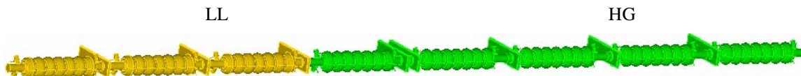
Figure 1: Eight cavities in the Renascence cryomodule. The first three are the Low Loss shape design and the remaining five are the High Gradient shape design. The locations of FPC couplers are mirrored about the middle of the cryomodule. Cavity 4 and 5 forms a back-back cavity pair. There are concerns of possible trapped modes in the FPC region.
