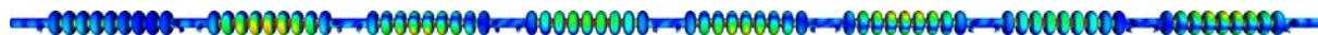
Figure 5. The electric field pattern of a trapped dipole mode inside an 8-cavity ILC cryomodule.
