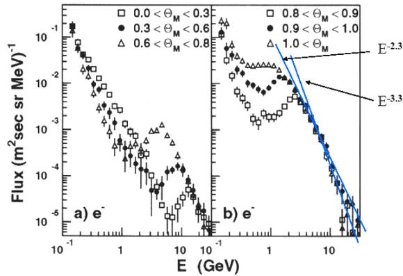
**FIGURE 2.** AMS electron spectra (Alcaraz et al. 2000, Aguilar et al., 2002). The break in spectral slope at  $\sim 7$  GeV corresponds to change between energy regions where diffusion and synchrotron losses dominate. Above this energy, the spectrum will continue with a constant slope until effects of nearby sources and diffusion in local magnetic fields become interesting above 1 TeV
