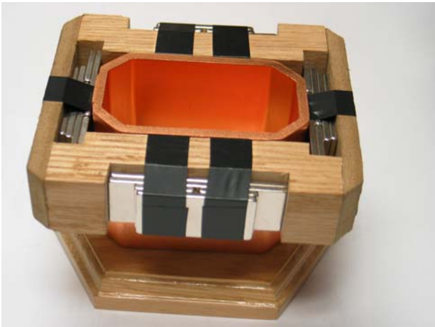
Figure 1: Prototype of permanent magnet skew quadrupole with 1.0 kG integrated strength.
