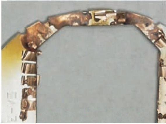
Figure 7: Damaged rf seal from a flex-flange connection.
