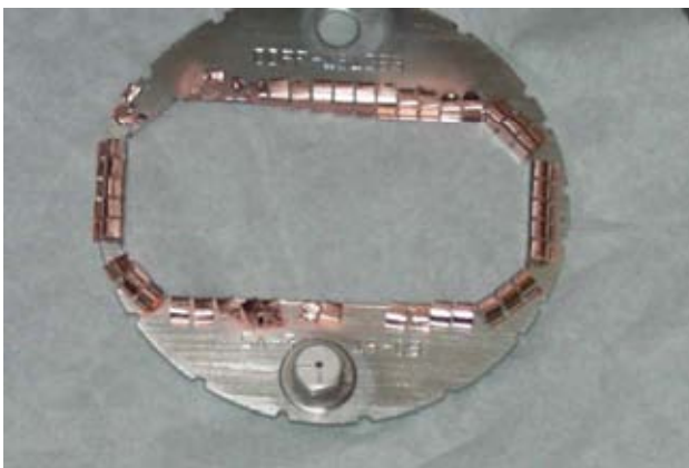
Figure 4. An RF seal designed to bridge the gap between two vacuum flanges. One can see that the stainless steel plate got hot enough to melt the copper (upper left corner) as well as vaporize the sliver plating on the mounting bolts and washers.
