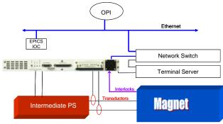
Figure 1: The Intermediate PS Architecture
