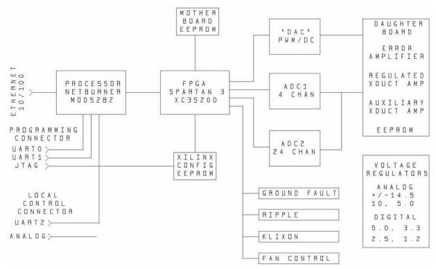
Figure 2: internal structure of the EPSC
