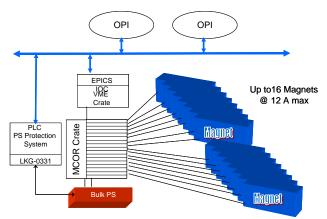
Figure 3: Bulk PS System Architecture - Magnets < 30A
