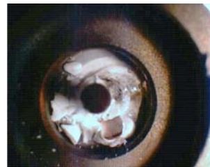
Figure 5: LER BPM feedthrough after overheating.
