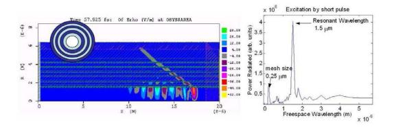
Figure 1: 2D simulation of the wake generated in a Bragg fiber. Left: Snapshot of  $E_r$  in the fiber. Note the Cherenkov angle within the bulk dielectric and the wake generated. The inset shows the cross-section of the fiber. Right: Fourier transform of the on-axis  $E_z$  field showing the resonance at the expected wavelength of  $1.5\mu$ m.
