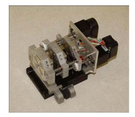
Figure 3: The Permanent Magnet Quadrupole triplet. The first two quads are movable by stepper motor to adjust the final focus, as is the assembly as a whole.
