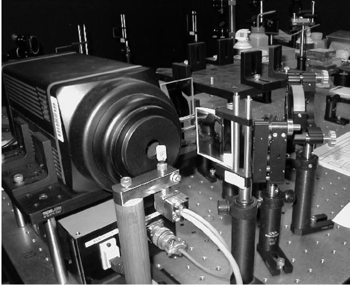
FIGURE 2. The galvanometer mirror, with its motor below, sits in front of the camera. At right, the final cylindrical lens.
