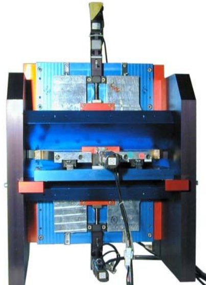
Fig. 1: Adjustable Strength PM Quadrupole
