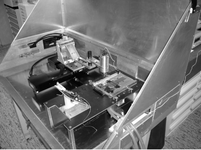
Fig. 3. Mechanical setup for the CCE measurements. The silicon module is mounted in a metal frame, and above it the brass cylinder holding the LED is clearly visible. The LED is moved above the detector surface by means of the black X - Y stage.
