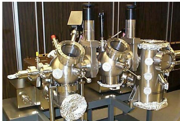
Figure 1: The photocathode deposition system used for CVD of cesium potassium antimonide photocathodes.
