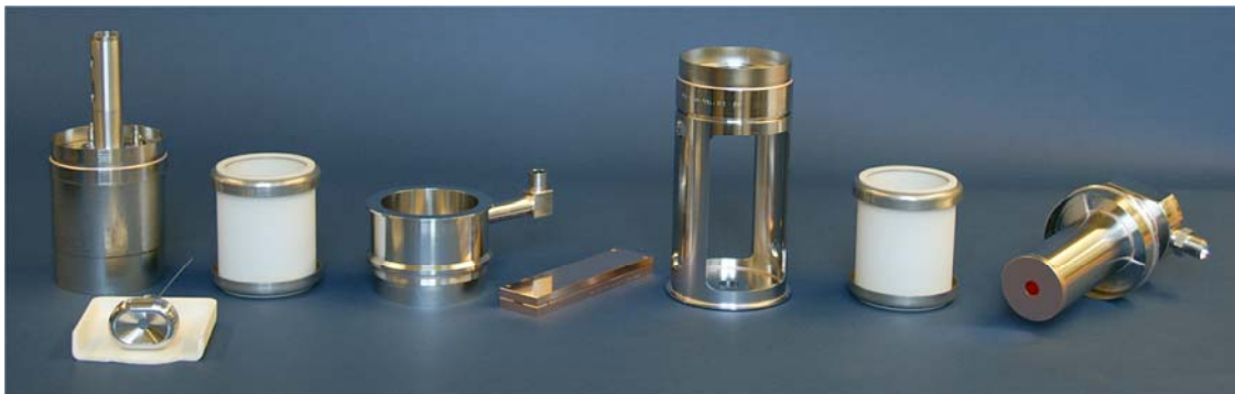
FIGURE 7. Photograph of the assemblies for the WSBK. The diffusion bonded copper circuit needs some final machining before the tube is assembled.
