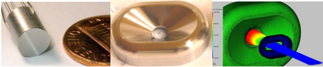
FIGURE 2. Photos of WSBK cathode and focus electrode with MICHELLE simulation output plot.
