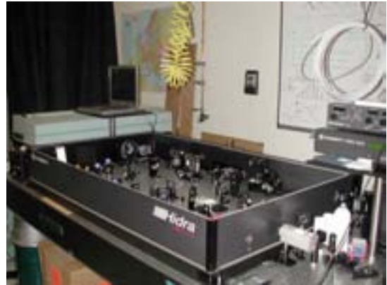
Figure 3: HIDRA-50 amplifier for the SPARC laser.
