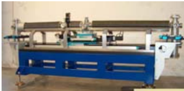
Figure 5: Emittance-meter device with long bellows.
