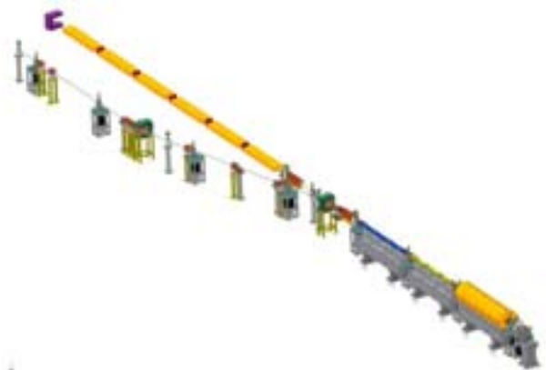
Figure 1: Layout of SPARC photo-injector, with RF-gun, 3 S-band accelerating sections and FEL undulator (6 modules). Beam line for undulator by-pass is also shown.
