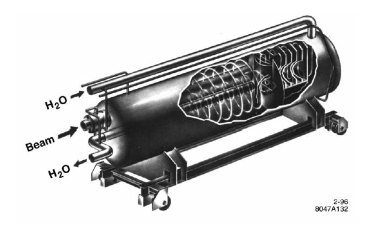
Figure 1: The water-based dump in use at SLAC [2]
