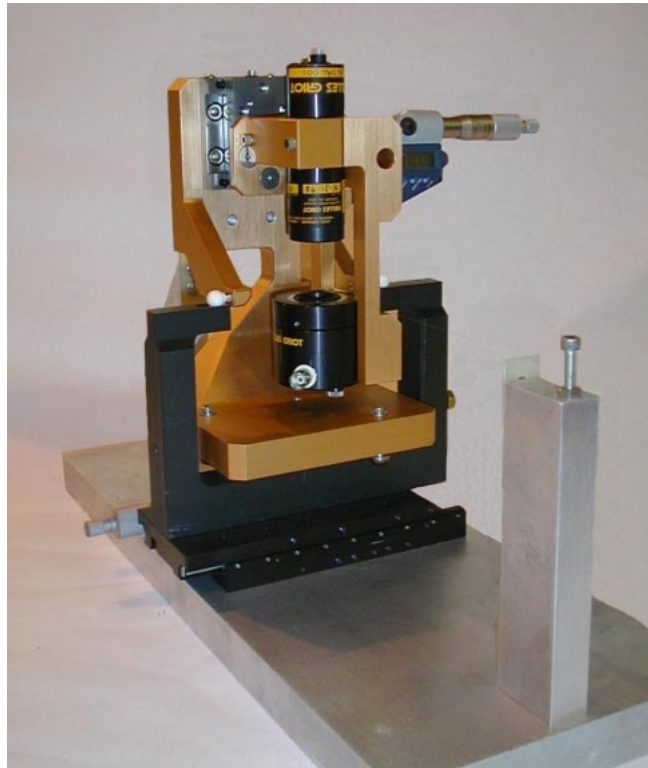
Figure 1- Wire Finder In Its Calibration Stand
