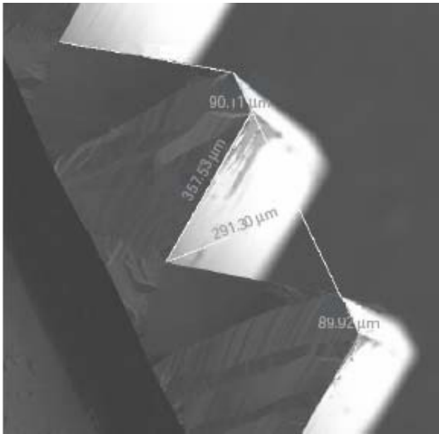
Figure 2: View of a 500 \mu\text{m} grating etched on (100) Si.
