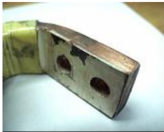
Figure 2: Silver Plating Came off
