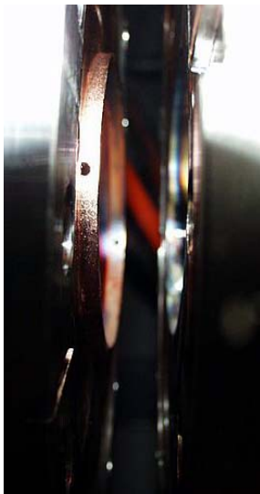
Figure 3: Photo of the disconnected stainless steel flanges and RF copper gap ring.
