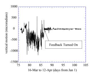
Figure 7. Signal from trajectory stabilization feedback.
