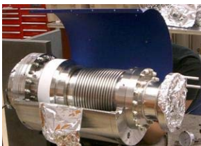
Figure 4: Low-impedance DCCT chamber.
