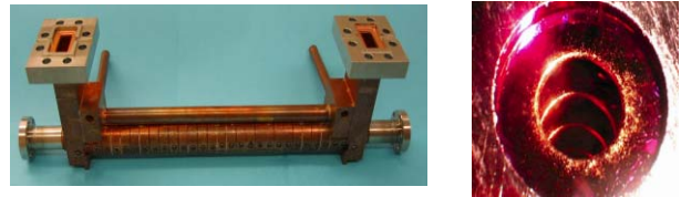
Figure 5. Damage in X-band structure.
