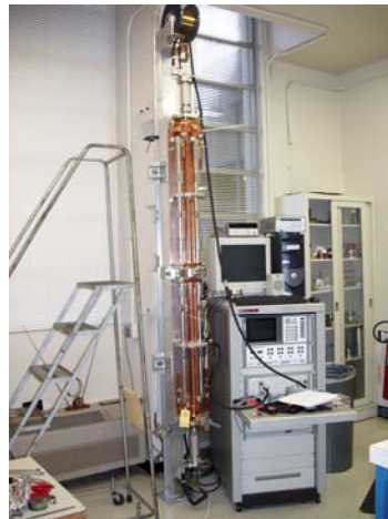
Figure 11: Wire measurement set-up with the RDDS1 structure.
