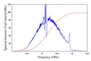
Figure 6b: Spectral function [10] as obtained from a circuit model [11]. The frequency errors in the middle of the spectrum, due to the deformation of the middle cells, are taken into account.
