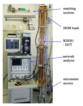
Figure 2: Wire measurement setup.
