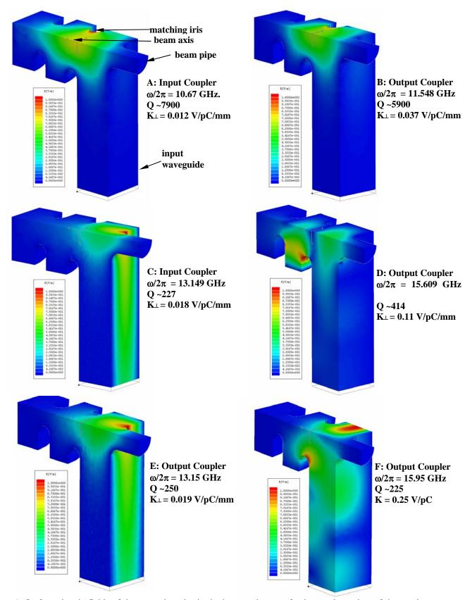
Figure 1: Surface electric fields of the trapped modes in the input and output fundamental couplers of the accelerator structure known as H60VG4S17-III-SN2. The resonant frequency  $(\omega/2\pi)$ , Q value and the dipole mode kick factor  $(\mathbf{K}_{\perp})$ , are indicated except for the monopole-like mode in F, where the monopole loss factor  $(\mathbf{K})$  is indicated. One quarter of the geometry was simulated with appropriate boundary conditions.
