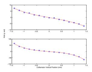
Figure 2: Kick angle vs collimator position. Top: Slot 1 (short Cu). Bottom: Slot 4 (long Ti).
