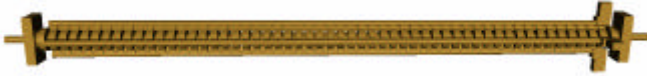
Figure 2: Model of the H60VG4 DDS structure with damping manifolds, input/output power couplers and HOM couplers.
