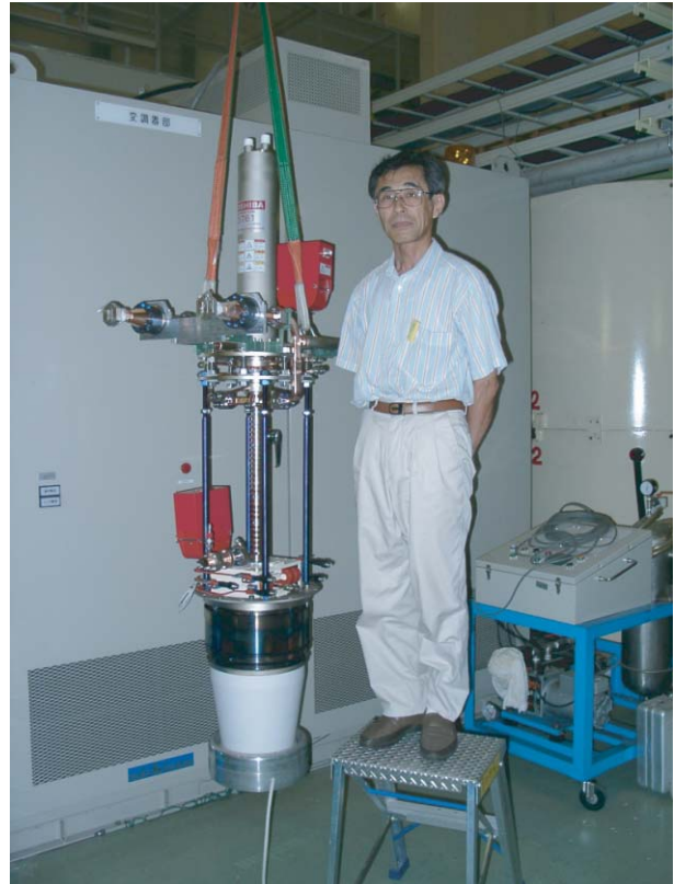
Figure 4: X-band PPM Klystron developed at KEK
