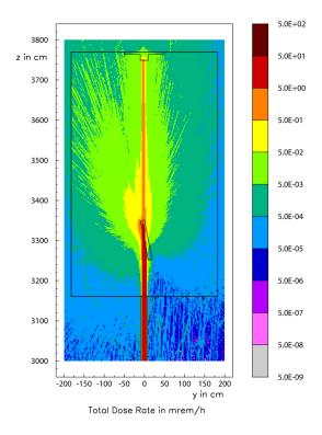
Fig. 12: Case 1 – Total dose rate at the experimental hutch. The beam is impinging on a Si-target.
