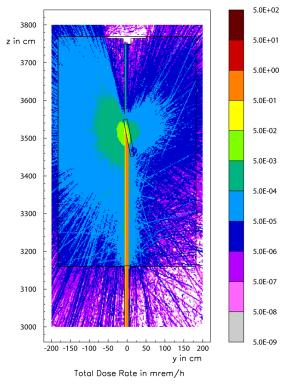
Fig. 16: Case 3 - Total dose rate at the experimental hutch. The x-ray beam is impinging on a Si-target.
