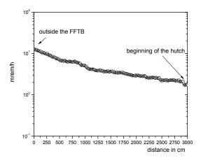
Fig. 9: Case 3 – Total dose rate in the center (1 cm diameter) of the beam pipe
