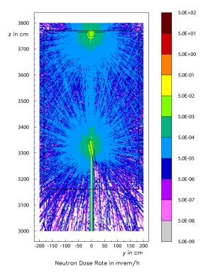
Fig. 15: Case 1 – Neutron dose rate at the experimental hutch. The beam is impinging on a Si-target.
