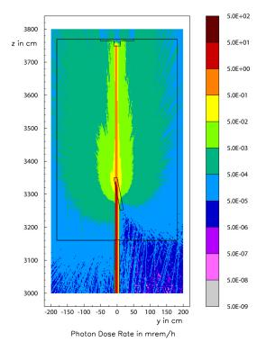
Fig. 13: Case 1 – Photon dose rate at the experimental hutch. The beam is impinging on a Si-target.
