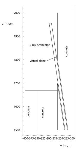
Fig. 5: Details of the FLUKA geometry at the location where the beam pipe exits the FFTB. The virtual plane is also shown where information of particles crossing the plane was written to a file for further processing.
