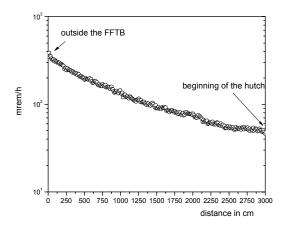
Fig. 8: Case 1 - Total dose rate in the center (1 cm diameter) of the beam pipe
