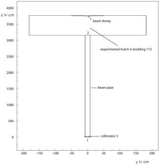
**Fig. 6**: FLUKA geometry of the beam pipe outside the FFTB and the experimental hutch.
