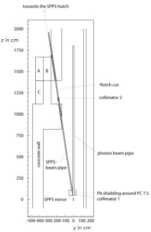
Fig. 4: FLUKA geometry of the FFTB – Horizontal sectional cut at beam height.
