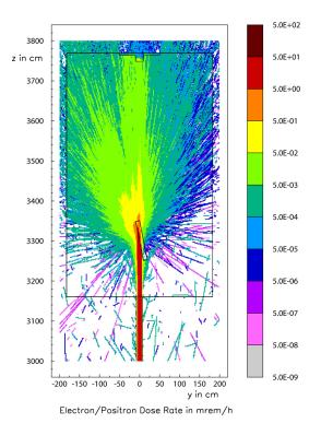
Fig. 14: Case 1 – Electron/positron dose rate at the experimental hutch. The beam is impinging on a Si-target.
