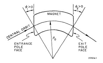
FIG. A-1--Field Boundaries for a bending magnet.
