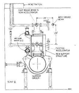
FIG. 2--Schematic of Accelerator Housing showing cross sections of present accelerator, 666 ft. new accelerator (east-bound beam) and return loop (west-bound beam).
