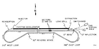
FIG. 1--Schematic layout of recirculation system.
