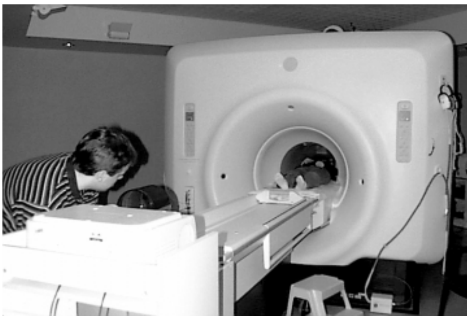
A 1.5 tesla MRI scanner at Stanford University for a functional neuroimaging study. The person in the foreground is adjusting a video projector used to present visual stimuli to the subject in the magnet. (Courtesy Anne Marie Sawyer-Glover, Lucas Center, Stanford University)
