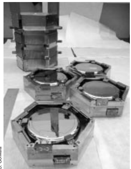
CDMS germanium detectors used in the 1999 run.
