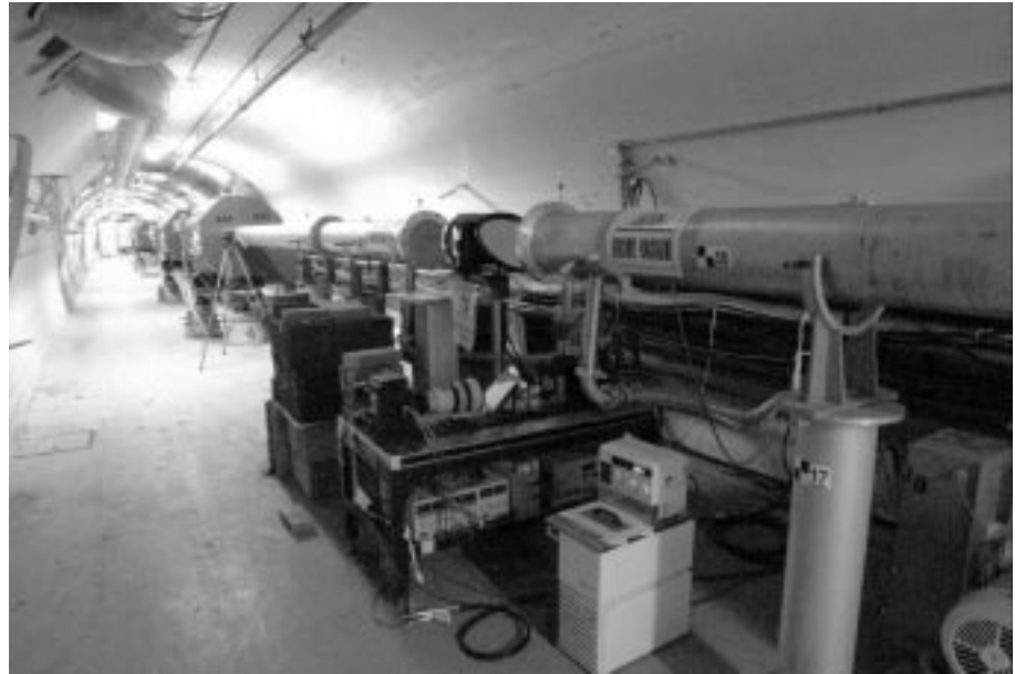
The E933 beam line at Brookhaven National Laboratory's Alternating Gradient Synchrotron. The view is looking downstream. The quadrupole magnets (octagon-shaped) are part of the first magnetic lens. The break in the beam pipe allows detectors to be set up at the first image station. Two camera systems are viewing the same scintillating fiber plane.
