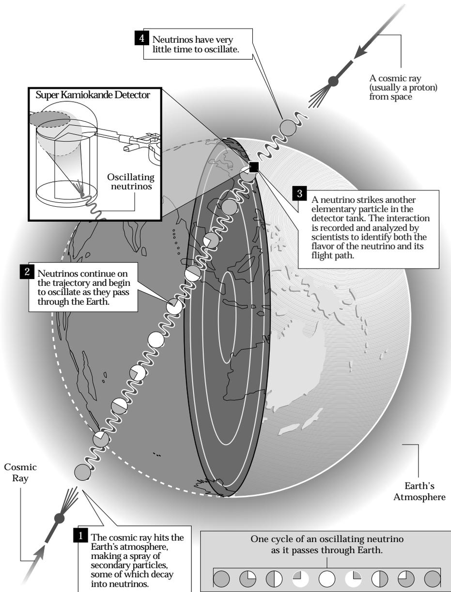
*A schematic illustrating the origin of neutrinos detected underground from high energy cosmic rays hitting the atmosphere and making secondary particles that decay, leaving neutrinos to penetrate the Earth and occasionally interact in detectors. The neutrinos coming from the far side of the world have much greater flight times during which to oscillate, as apparently do muon neutrinos but not electron neutrinos. (Courtesy University of Hawaii)*
