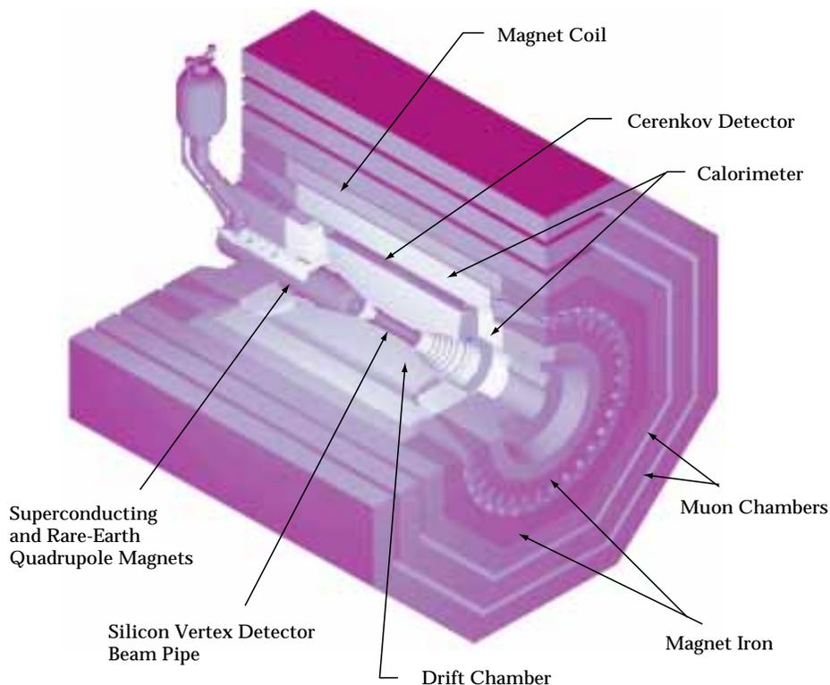
*A cutaway view of the CLEO III detector. The calorimeter, magnet, and muon system are preserved from CLEO II. The Cerenkov detector, drift chamber, and silicon detector are new. Also shown are the new CESR superconducting and rare-earth quadrupole magnets that are part of the machine upgrade.*
