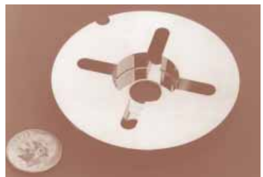
Cutaway view of part of a damped and detuned accelerator structure (top). The structure is fabricated from a stack of cells similar to the one shown above.
