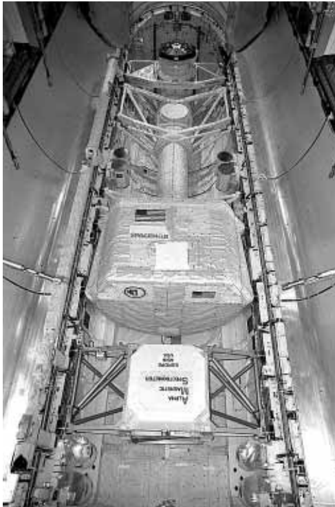
The AMS module installed in the Space Shuttle's payload bay. Above is the Spacehab module with supplies and logistics for the Russian Mir space station. This Discovery mission was the last of nine such dockings with Mir.
