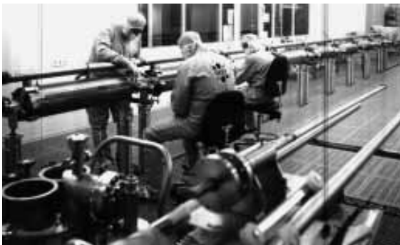
Assembly of the first string of eight TESLA cavities in the clean room at the Test Facility. (Courtesy DESY)
