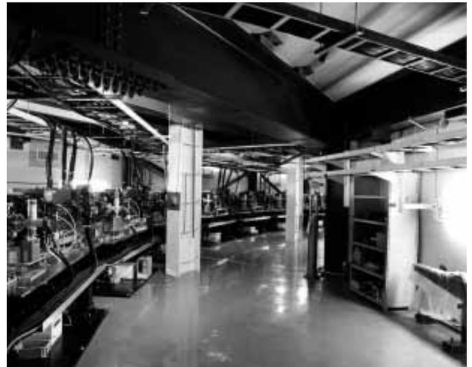
*Damping ring in the Accelerator Test Facility at KEK.*
